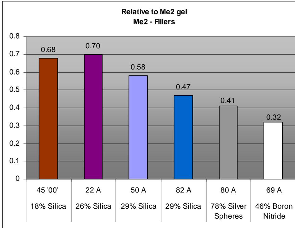
**Figure 6: Relative Permeability Rates of filled systems Silica, Silver, Boron Nitride**
