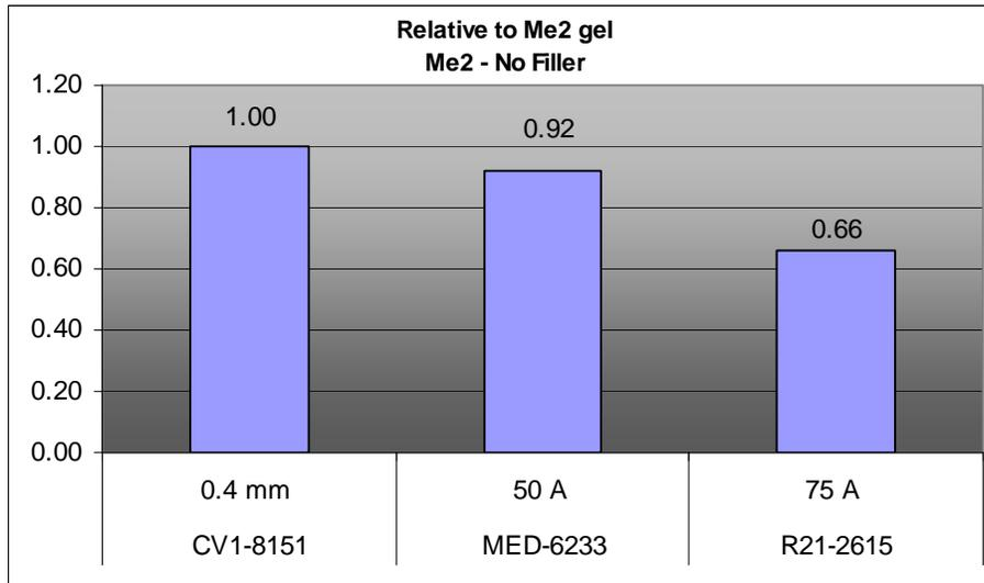
**Figure 7: Relative Permeability Rates of PDMS to Me2 Gel: No Filler, Different Hardness**
